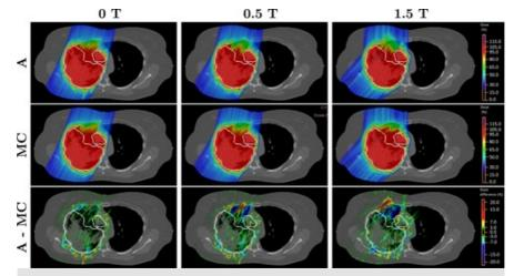
Treatment plan for lung patients optimised for 0 T (left), 0.5 T (centre) and 1.5 T (right). Dose distributions calculated analytically (top), with TOPAS-MC (middle) and their difference (bottom) are shown.
