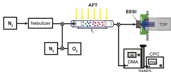
**Fig. 1:** Aerosol flow tube setup coupled to an EESI-TOF-MS and SMPS system.
