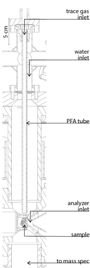
**Fig. 1:** Sketch of the ISS endstation showing the inert fluoropolymer (PFA) tube for trace gas dosing and the location of the mass spectrometer inlet.
