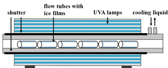
**Fig. 1:** Set-up of the CWFT experiments, with six short tubes coated inside with ice films and placed inside the cooled glass reactor, surrounded by seven UVA lamps for irradiation. The black cover to shield the flow tubes from the light before starting the experiment, is indicated as « shutter ».
