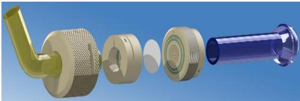
**Fig. 1:** The illustration shows an exploded view of the filter unit with all associated compression-fitting parts.
