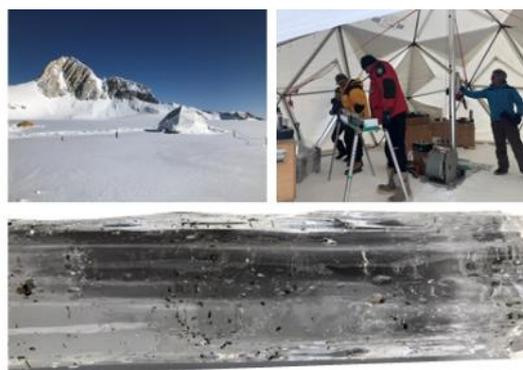
**Fig. 2:** Drill location and inside of the drill tent (top). Bottom most ADA270 ice core section. Note the crystal-clear ice (no dust from mechanical drilling) allowing to visibly recognizing ice crystal size and larger particles (dust/rocks, organic fragments).
